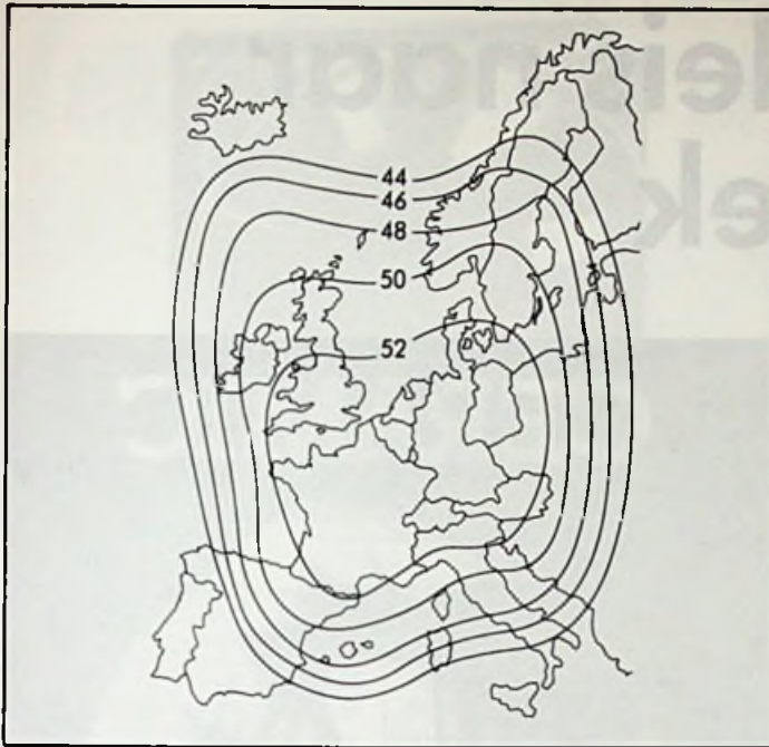
Astra 1A Spot Beam, 19,2° oost, horizontale polarisatie (in dBW).
